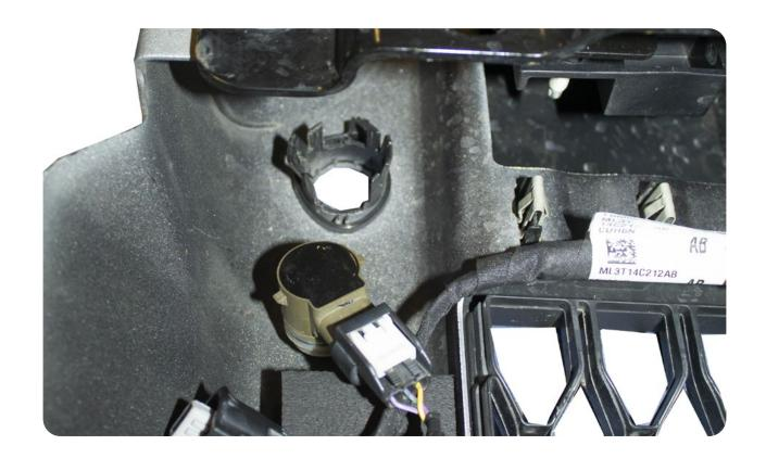
Spread these two tabs to release the sensor from its mounting ring.
