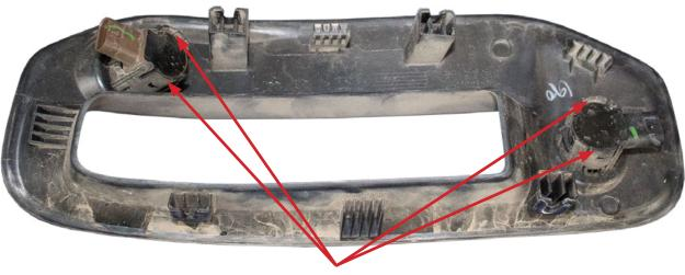
Spread these tabs to release the parking sensors
