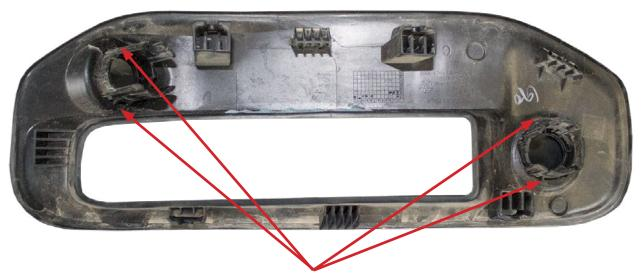
Squeeze these tabs to release the sensor mounting rings
