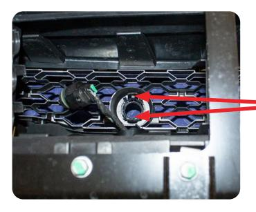
Squeeze these two tabs to release the mounting rings from the bumper
