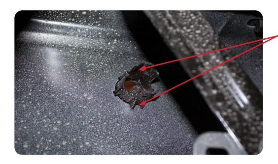
SQUEEZE THESE TWO TABS TO RELEASE THE PARKING SENSOR MOUNTING RINGS.
