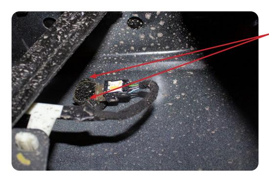
SPREAD THESE TWO TABS TO RELEASE THE PARKING SENSOR.
