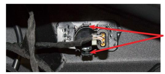
Spread these tabs to release the sensor
